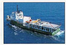
Western's purpose-built 4-D/4-C OBC fleet can deploy the energy source, cable, and recording equipment from a single vessel. This versatile package allows Western to mobilize quickly and economically for targeted 4-D/4-C surveys.
